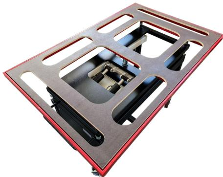
The TECHNIQUE T3300 non-conductive wooden loading platform top incorporates specially designed shapes to help facilitate the operators access when working underneath the vehicle. This enables easy working and access to components, battery packs, engine transmissions and motors. The user can walk within the lifting space to further help the user with dismantling operations.
